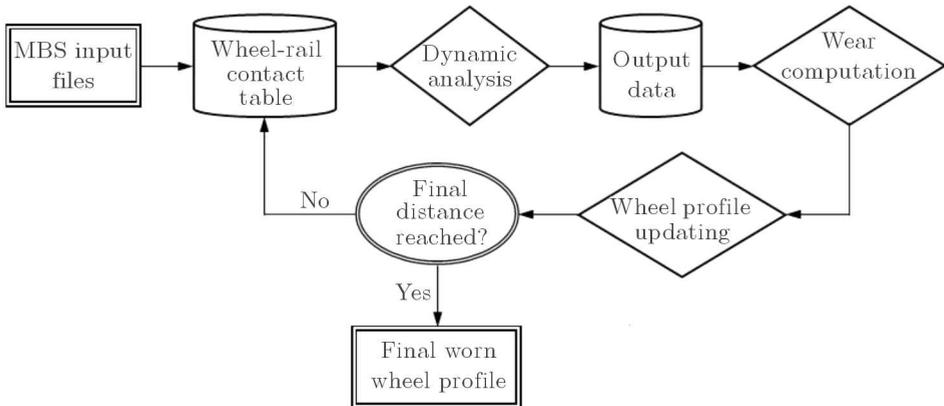
Fig. 1. Schematic representation of the wear prediction tool
