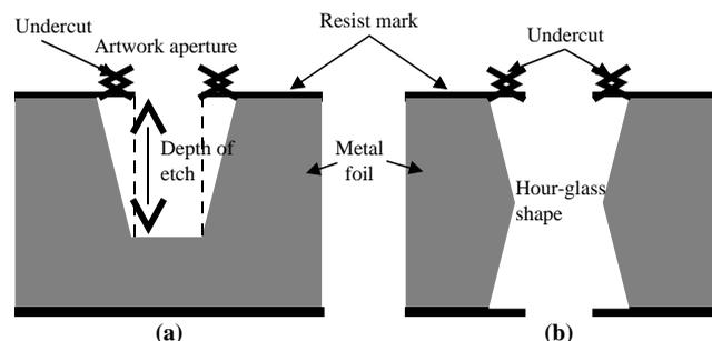
Notes: (a) Etching one side of the metal foil; (b) etching on both sides of the metal foil
