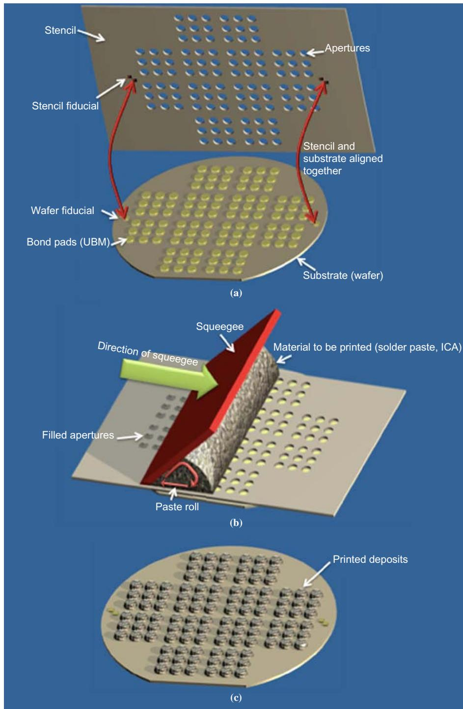
**Notes:** (a) Stencil and substrate are aligned together; (b) substrate is brought in close proximity or contact with the stencil and the squeegee is driven across the stencil surface, as the printing material passes the apertures it fills them; (c) substrate is separated from the stencil and the contents of the apertures are transferred onto the substrate
